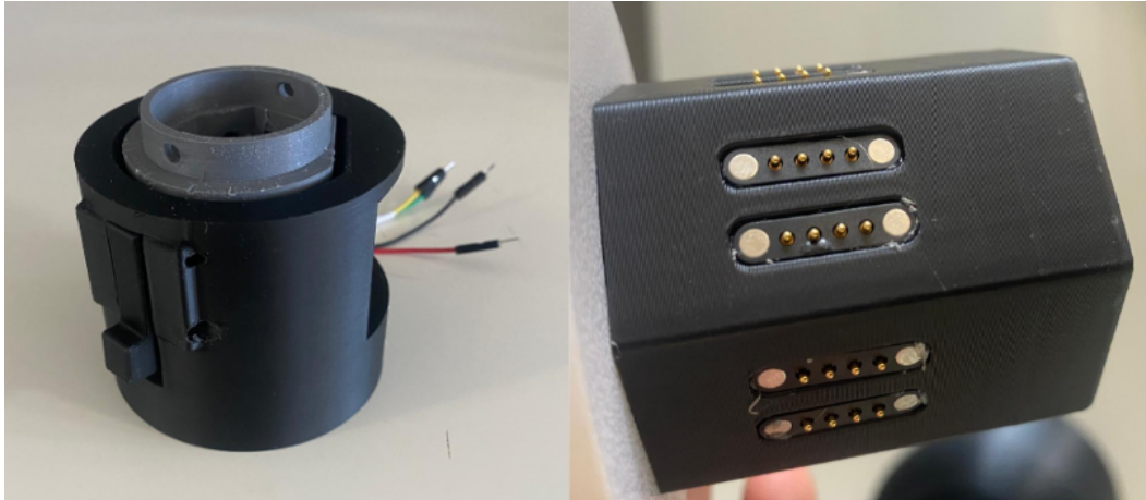
Figure 5.7: Final prototype of the developed coupling system showing the socket (left) and the connector with the integrated pogo-pin interface (right)
