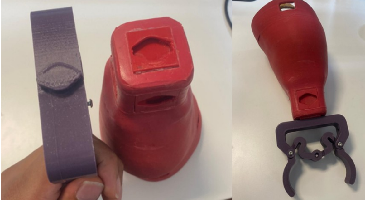
Figure 2.6: Examples of mechanically interchangeable prosthetic gadgets and coupling interfaces used in the eSuperheroes project
