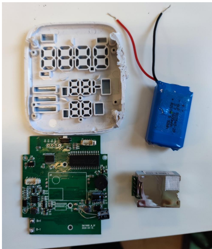
Figura 2.8.- Despiece del sensor CO 2 TACKLY.
