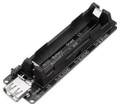
Figura 3.8.- Battery shield 18650
